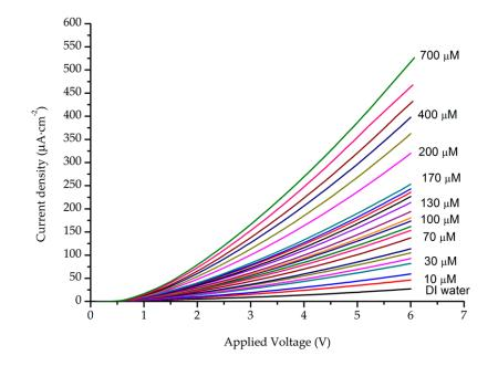
**Figure 2.** I-V characteristics of the ZnO NR sensing electrode for  $H_2O_2$  in concentrations ranging from 10  $\mu$ M to 700  $\mu$ M.
