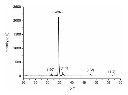
Figure 1. The XRD pattern of the prepared ZnO NRs on the AZO substrate.
