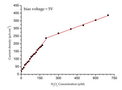
**Figure 3.** Response of the AZO/ZnO NR sensing electrode at bias voltages of 5 V in a diluted solution of  $H_2O_2$  in concentrations ranging from 10  $\mu$ M to 700  $\mu$ M.
