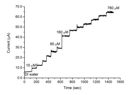
**Figure 4.** The amperometric response of the ZnO NR/AZO electrode upon successive additions of  $H_2O_2$ . The bias voltage was fixed at 5 V.
