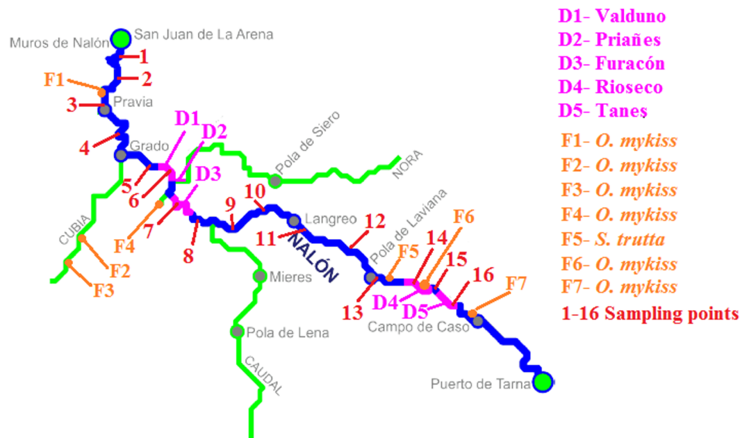
Figure 2 Nalón River basin. Dams along the river are shown; from downstream to upstream they are Valduno (D1), Priañes (D2), Furacón (D3), Rioseco (D4) and Tanes (D5). The fish farms are pointed as F1 to F7 and finally the sampling points are numbered in red from 1 to 16.
