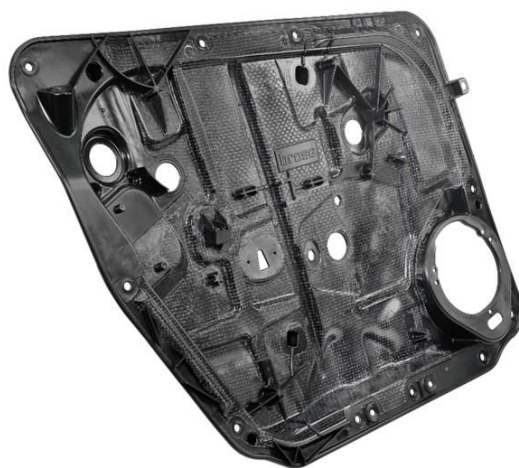
Figure 1. Typical door module carrier hybrid-component made of polypropylene with woven-glass-fiber-reinforced organo sheet and injected with structures (ribs, functional elements, edges, etc.) Reprinted/adapted with permission from Ref. [9]. 2021, ElringKlinger.
