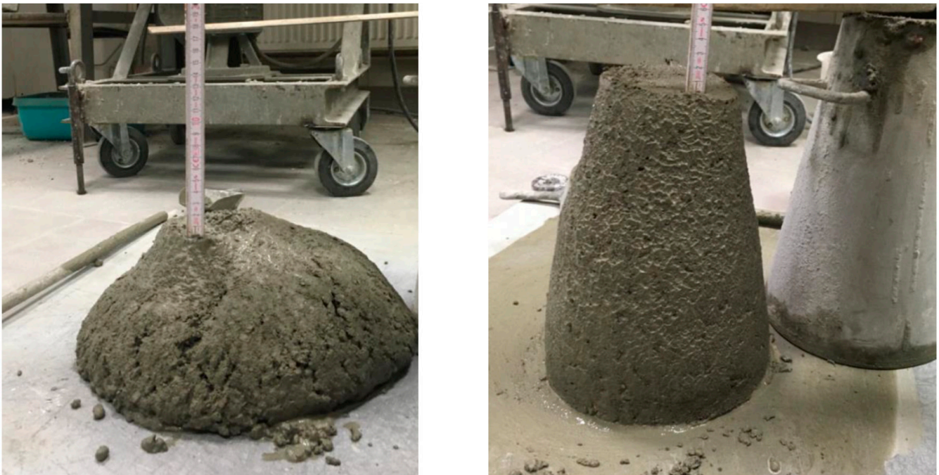
Figure 5. Photograph of the difference in consistency measured with the slump test method between the REF 1 series (left photo) and SAP SH50 (right photo).
