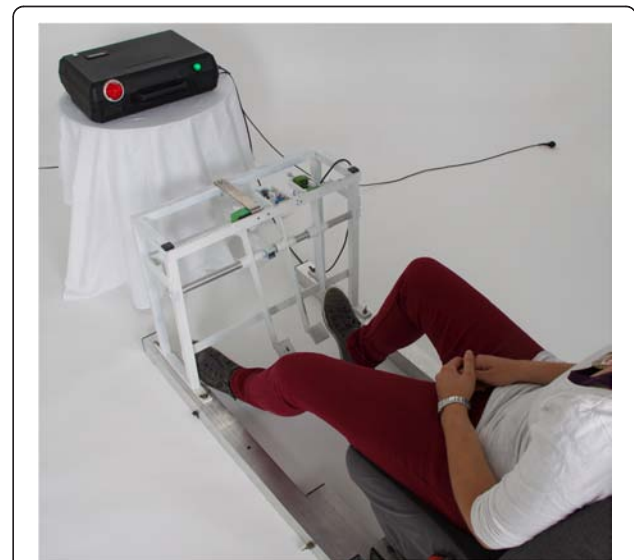
Fig. 1 Custom-made apparatus for measuring brake response time (BRT). Pedals from left to right: coupler [clutch] pedal; brake pedal; accelerator pedal. External box: red light (visual stimulus initiating the braking procedure); green light (indicating that the accelerator is fully depressed—subject not in a 'ready-to-brake fashion')
