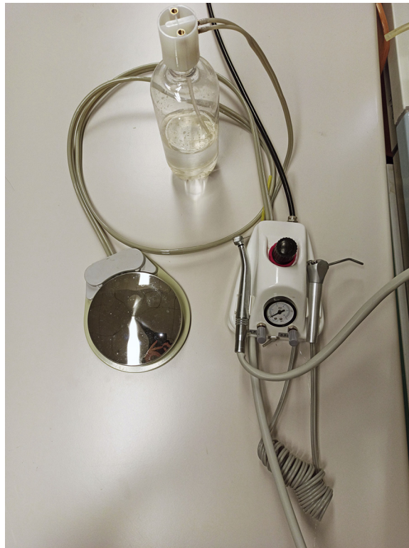
Figure 2. The air turbine and control apparatus used in the study. The pressurized water tank used to generate the air-water cooling spray for the turbine handpiece is seen at the top of the photo.
