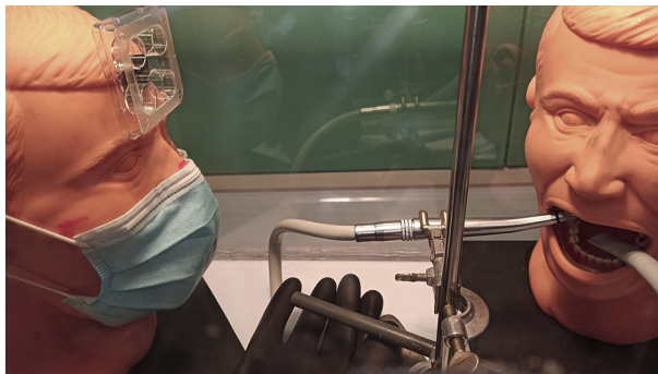
Figure 3. The 2 manikins inside the chamber. On the right, the patient manikin can be seen with the air turbine and high-volume evacuation tip fixed in the same position throughout all experimental runs, as if operated by a right-handed dentist and dental assistant. On the left, the operator manikin is equipped for the first experimental run. In all runs, the chamber space between operator and patient manikins was free of materials and gloves to allow for an even aerosol spread, similar to clinical conditions.
