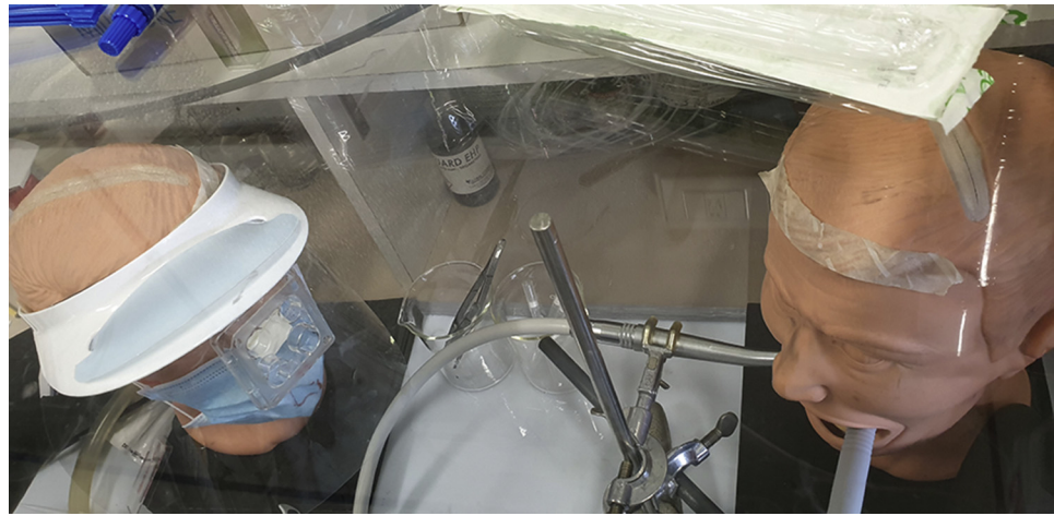
Figure 6. The setup for the fifth experimental run, testing the association of face shield and surgical mask, is visible through the transparent upper panel of the chamber. The forehead target was fixed to the upper external part of the face shield.
