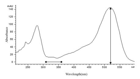
**Figure 2.** UV-Vis spectrum of the primary peak. The maximum absorbance at 520 nm. The lack of absorbance in the region between 310 and 360 nm (horizontal bar) indicates that the compound might not be acylated.
