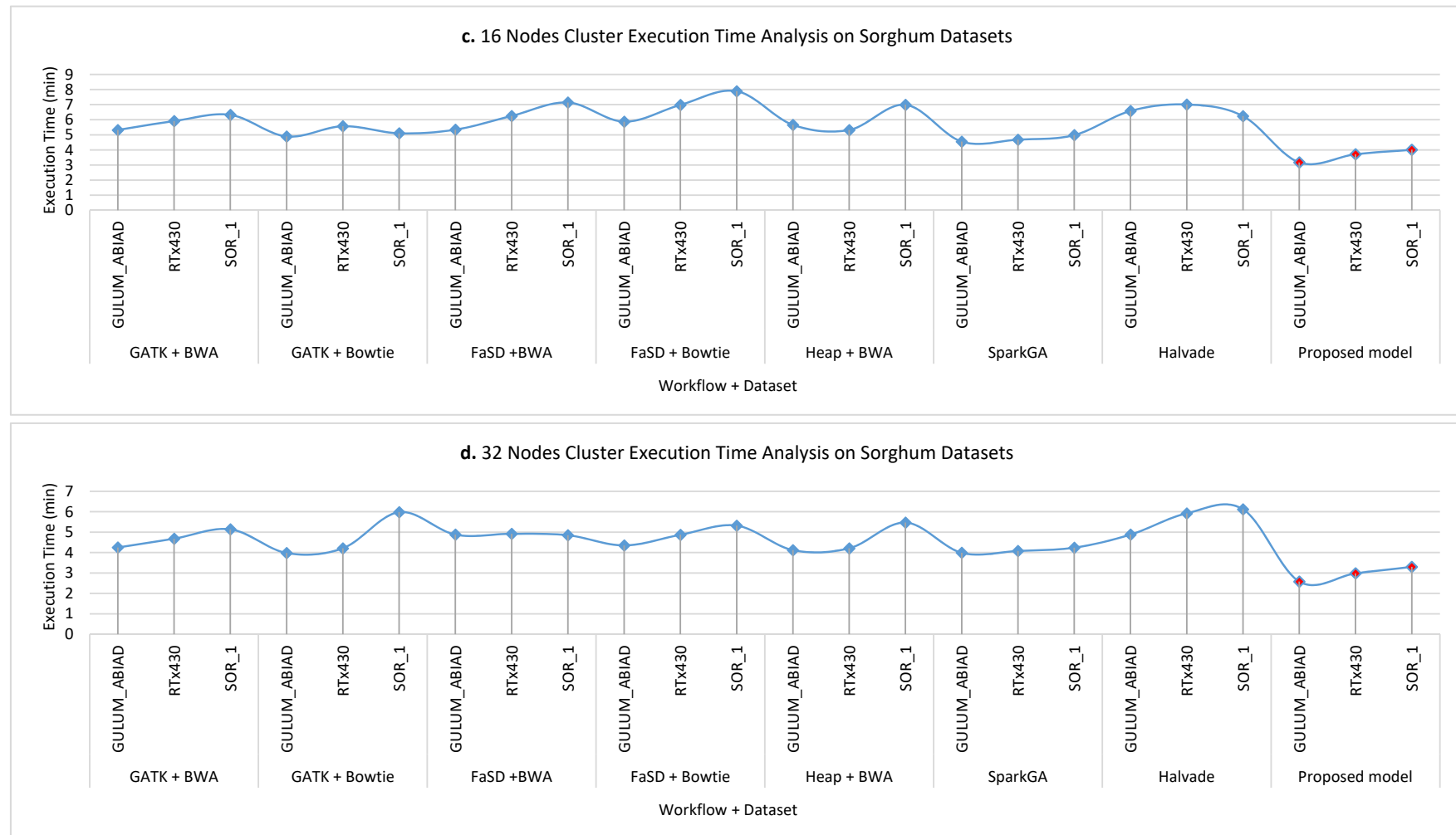
Figure 7. The execution time analysis of single node pseudo cluster, 8 nodes, 16 nodes, and 32 nodes real clusters are shown in part (a–d) respectively for Sorghum datasets. The light blue filled circle markers over the line show the values for existing workflows and the solid red filled circle shows the values for the proposed workflow. Here, it is clear that the proposed workflow takes less time in execution for detecting SNPs as compared to others. It is worth noting that on a larger dataset the efficiency of the proposed framework is much better than a smaller dataset.
