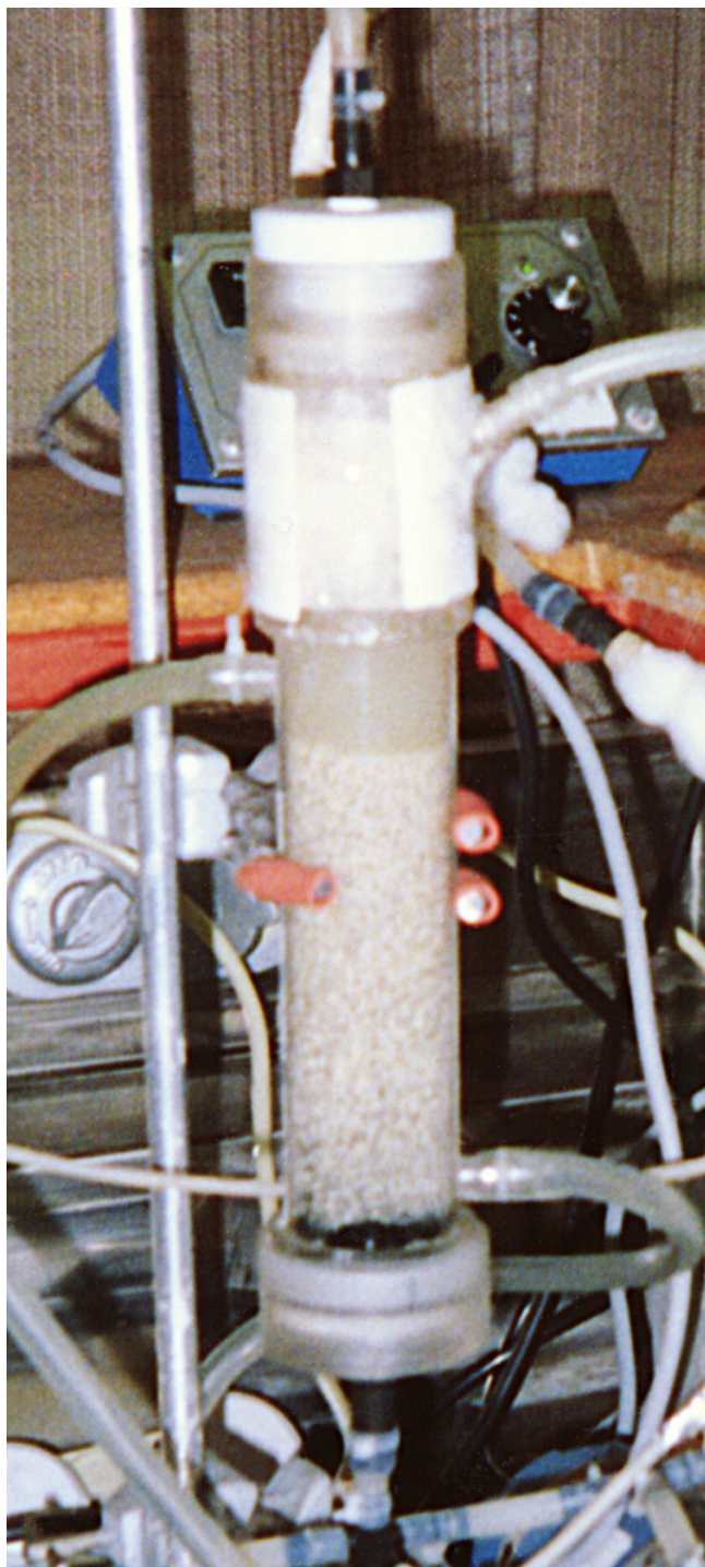
Figure 5 A photograph of a fluidized bed bioreactor (inside volume 450 cm 3 ) used to produce butanol from whey permeate using C. acetobutylicum P262.
