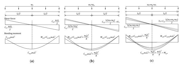
**Figure A2.** Failure mechanism for DB-1 region. (a) Flexural failure at the N2 section first; next, (b) flexural failure at the N1 section; and finally, (c) shear failure at the N2 section.
