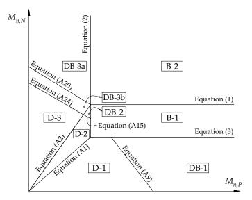
**Figure 4.** Different failure modes according to  $M_{n,P}$ ,  $M_{n,N}$ , and  $V_n$  for the end span of an RC slab.
