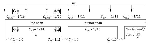
Figure 2. Moment and shear coefficients for continuous RC slabs with column supports reported by ACI 318M.
