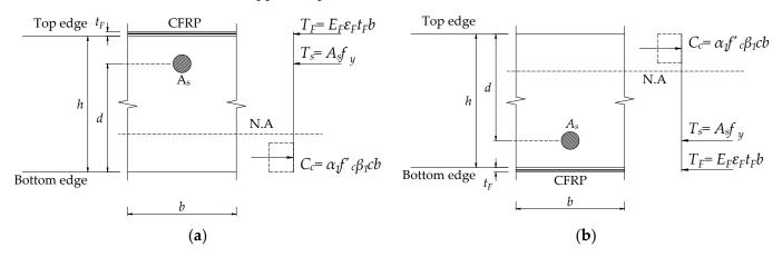
Figure 5. The CFRP strengthened sections are subjected to (a) negative moment and (b) positive moment.
