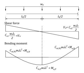
**Figure A9.** The failure mechanism for B-2 region; shear failure at N2 section without forming any plastic hinge.
