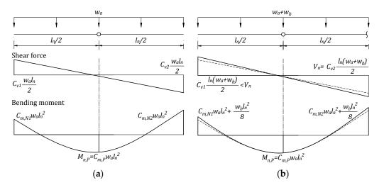
**Figure A6.** Failure mechanism for DB-3a region. (**a**) Flexural failure at the mid-span section first and then (**b**) shear failure at the N2 section.
