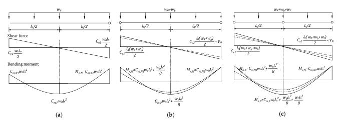
**Figure A1.** Failure mechanism for D-1 region. (**a**) Flexural failure at the N2 section first; next, (**b**) flexural failure at the N1 section; and finally, (**c**) flexural failure at the mid-span section.
