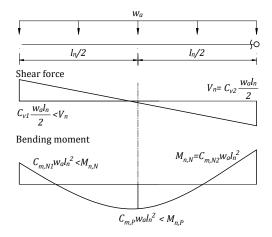
**Figure A8.** The failure mechanism for B-1 region; shear failure at N2 section after forming a plastic hinge at the N2 section.
