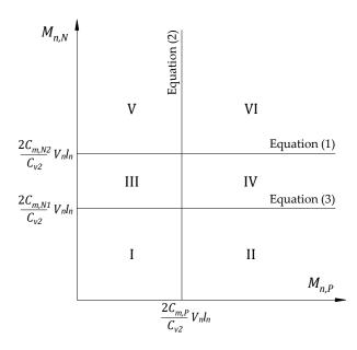
**Figure 3.** The failure regions are described considering the relationship between the shear limit and moment limit of the slab sections.
