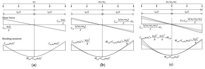
**Figure A7.** The failure mechanism for DB-3b region. (a) Flexural failure at the mid-span section first; next, (b) flexural failure at the N2 section; and finally, (c) shear failure at the N2 section.
