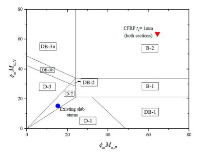
Figure 6. Failure limits for the flexural strengthened slab with CFRP.
