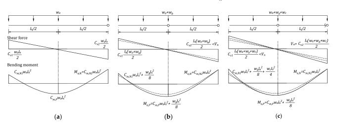
**Figure A4.** Failure mechanism for DB-2 region. (**a**) Flexural failure at the N2 section first; next, (**b**) flexural failure at the mid-span section; and finally, (**c**) shear failure at the N2 section.
