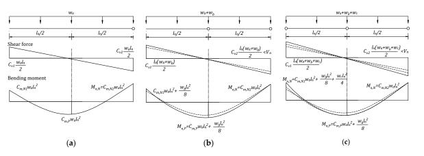
**Figure A3.** Failure mechanism for D-2 region. (**a**) Flexural failure at the N2 section first; next, (**b**) flexural failure at the mid-span section; and finally, (**c**) flexural failure at the N1 section.
