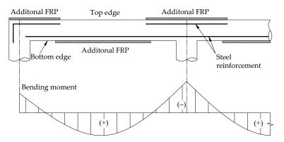
Figure 1. Externally bonded FRP strengthened slab at conventional locations.
