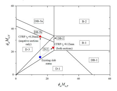
Figure 7. Failure limits for the flexural strengthened slab with CFRP considering ductile failure.
