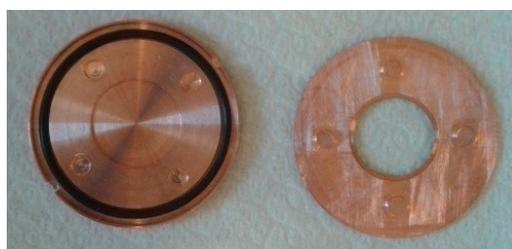
**Figure 2.** Four-pin clamping target system.
