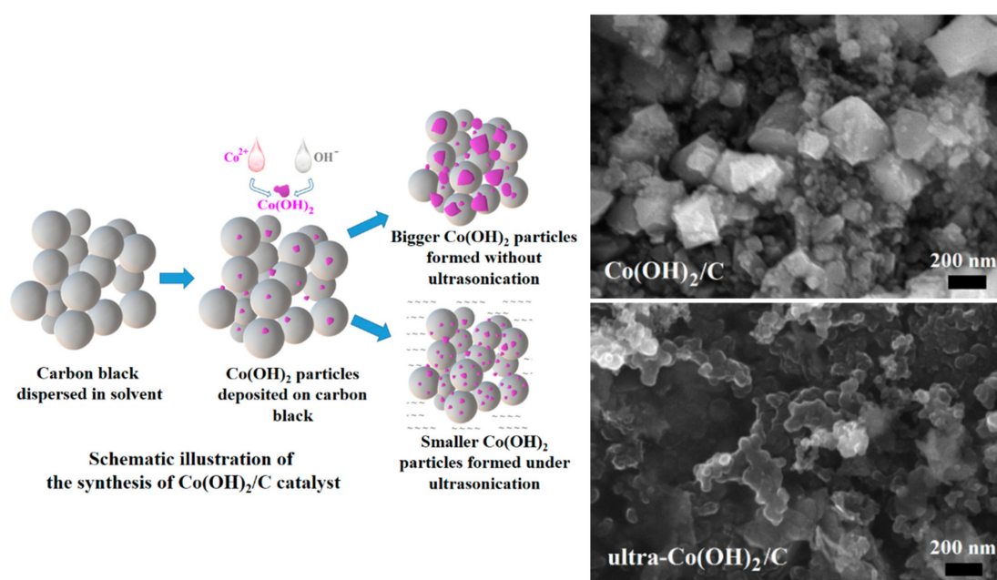
Figure 1. Fabrication of \text{Co}(\text{OH})_2/\text{C} , ultra- \text{Co}(\text{OH})_2/\text{C} and the scanning electron microscopy (SEM) images of the catalysts.
