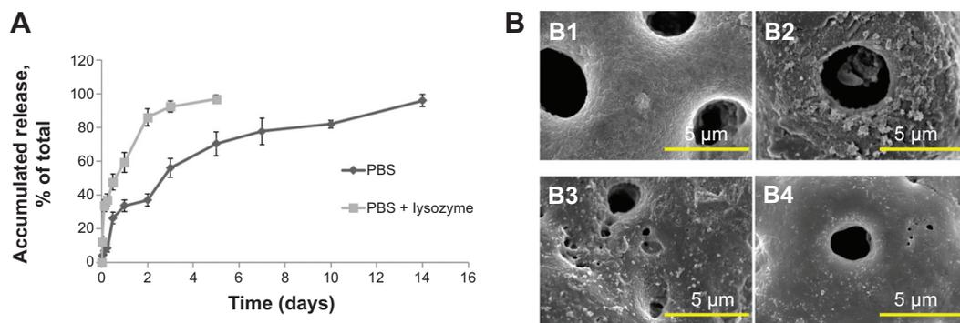
**Figure 2** Accumulated release profile of CS/Sema-MAO in PBS and PBS + lysozyme (**A**) and the morphology observation of the substrate after 1 day (**B1**), 3 days (**B2**), 7 days (**B3**), and 14 days (**B4**) of dissolution in PBS.
