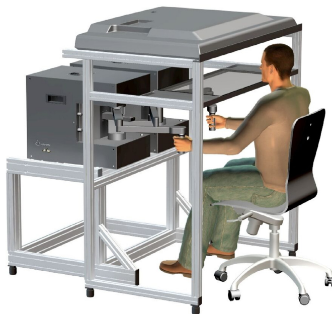
Figure 2 Three-dimensional animated representation of the KINARM endpoint robotic set-up used at 3 and 12 months follow-up assessments.
