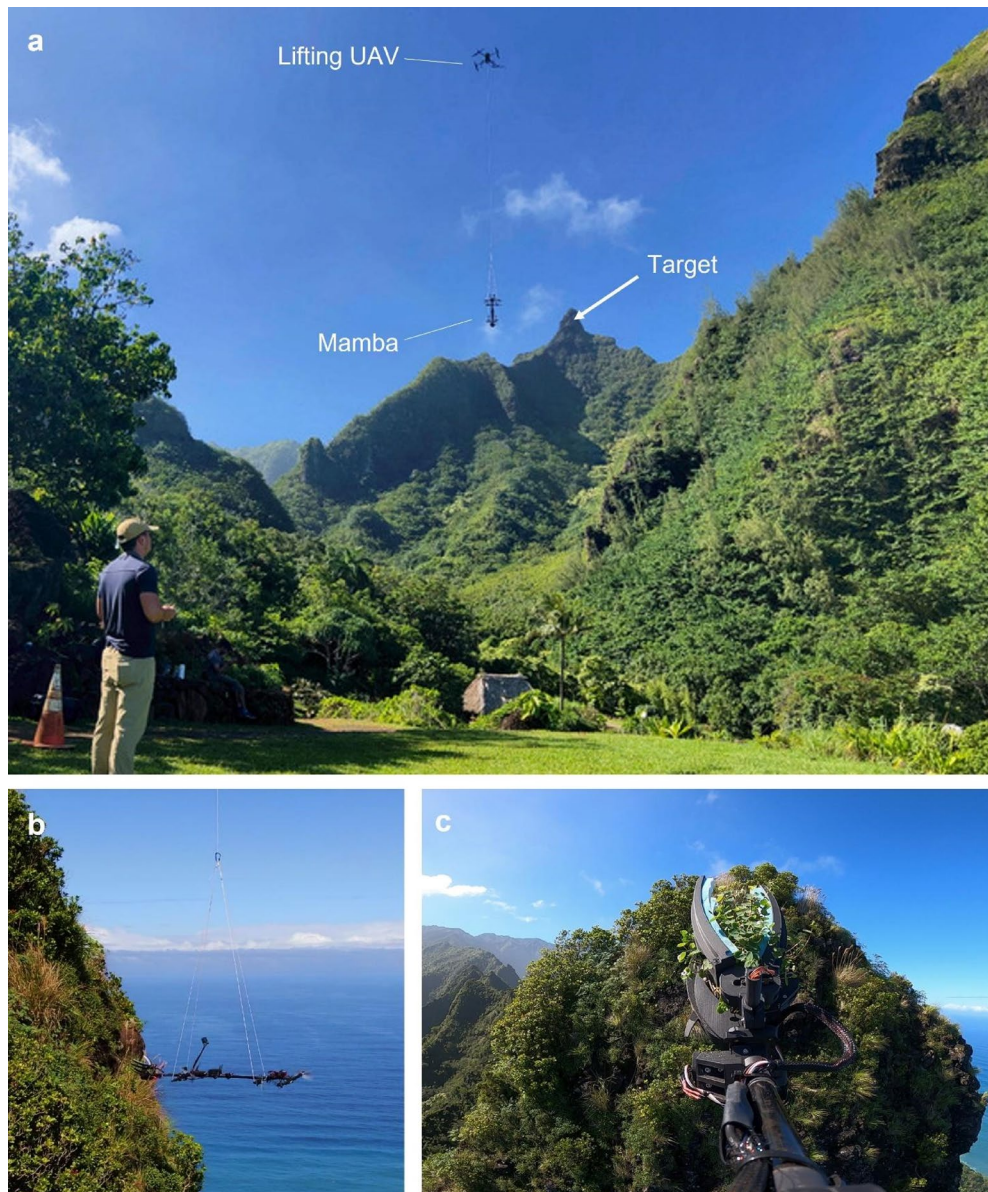
Figure 1. Aerial photos of the Mamba system during a mission at Limahuli Garden, Kauai, to collect Euphorbia elaeagnifolia . (a) Takeoff and travel to the target, located 1 km away from the base station. (b) Final approach on the target using the Mamba control system. (c) View as seen from the pilot from a first-person view camera with the sample secured in the tool.
