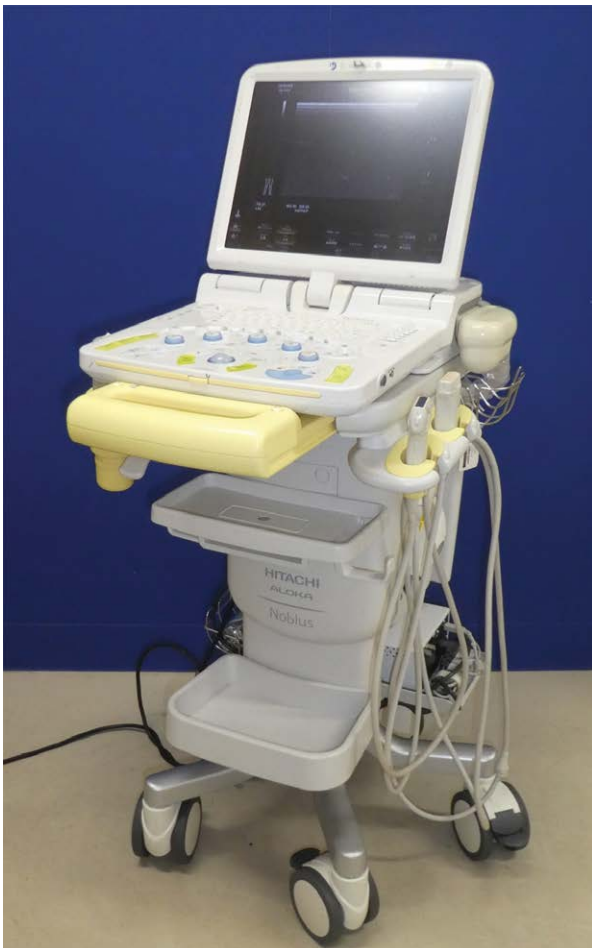
Fig. 1. Ultrasound device used for lymphatic ultrasound. No special probe is necessary for lymphatic ultrasound, and it can be performed using ultrasound device and linear probes found in general medical facilities.
