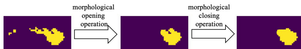
Figure 3 Noise cancellation and missing pixel filling based on numerical morphology.
