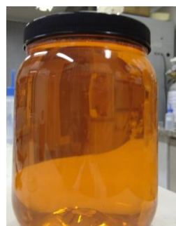
Figure 9. Cylindrical vial (20 cm tall and 15 cm in diameter) filled with FXO-f to perform 3D dosimetry.
