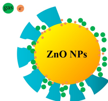
Figure 17. Schematic diagram of the ZnO@ZIF-8 composite with incomplete coating.
