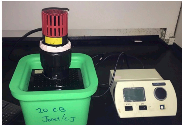
Figure 3. Exposure of sample to UV lamp in 96 well plate (black, clear bottom) on top of ice
