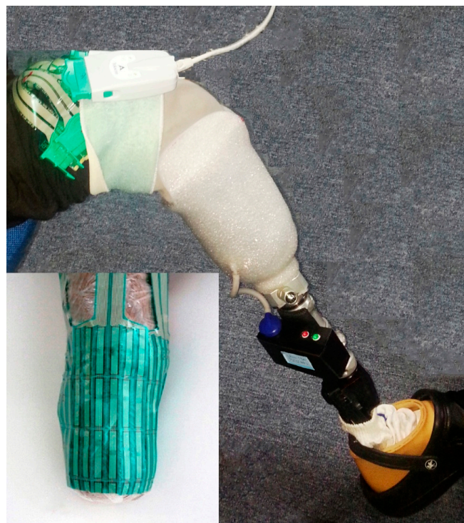
Figure 5. F-Scan test setup.
