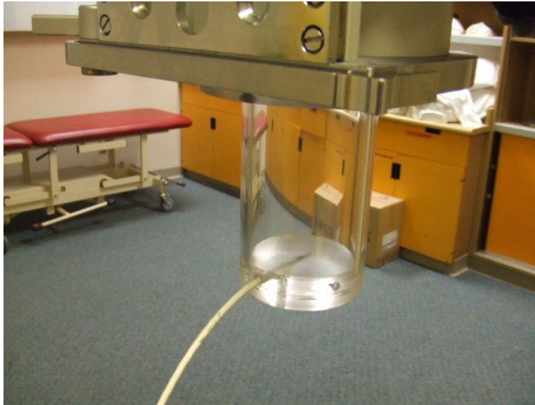
FIG. 2. The ion chamber and holder were used for output consistency check
