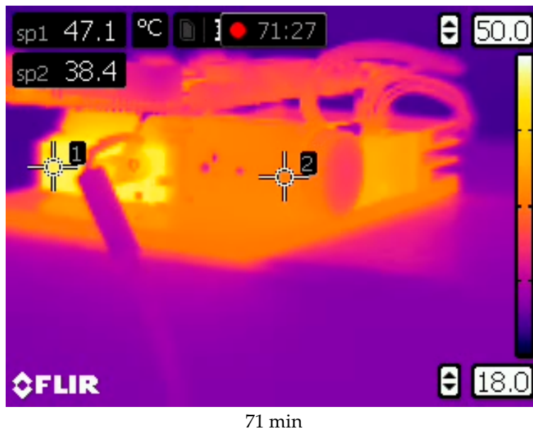
Figure 3. The warming-up process of the DLP LightCrafter 4500 projector, registered with thermal camera Flir E40. The colors on the presented images show the projector temperature in the first 71 min after turning on the power supply. The LED source is the warmer place on the projector (measuring point sp1).
