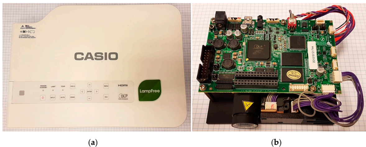
Figure 1. The projectors used in the experiments: (a) business-class projector DLP Casio XJ-A252; and (b) development kit projector DLPLightCrafter 4500.
