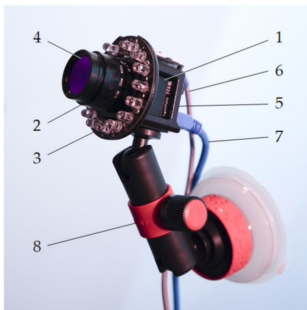
Figure 1. Main hardware components of the detector: 1—camera body; 2—lens; 3—IR illuminator; 4—band-pass filter; 5—supporting frame; 6—illuminator control cable; 7—camera data cable; 8—ball-joint holder.
