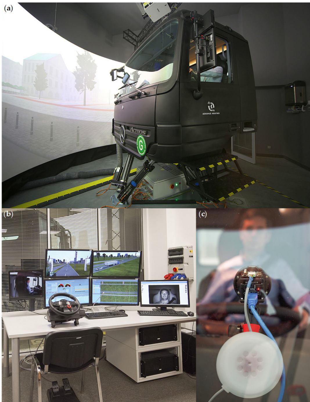
Figure 3. Photograph of the simulator system: the (a) exterior of the truck cabin, (b) instructor room, and (c) detector attached to the front window and directed towards the driver's face.
