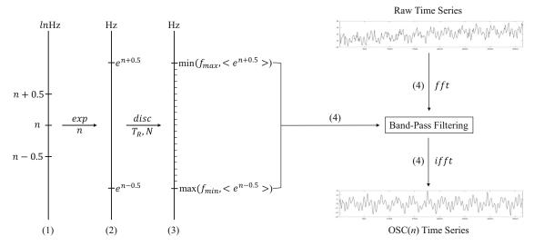
**Fig. 1** The flowchart on the DREAM algorithm. (1) N3L theory defines an oscillator with a length-one frequency band centered at n, i.e., OSC(n), in the natural log space. (2) In original frequency space, it expands the frequency band ( $e^{n-0.5}$ ,  $e^{n+0.5}$ ) Hz. (3) This frequency
