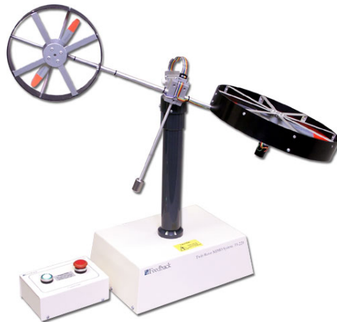
Figure 1. Twin rotor MIMO system (TRMS).
