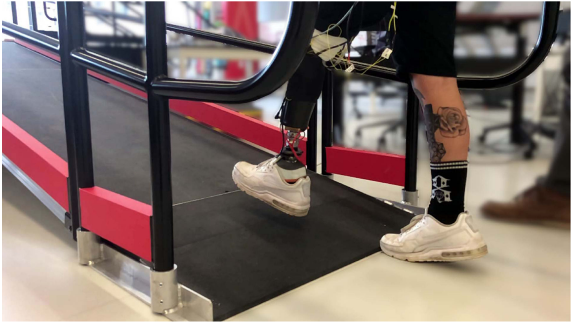
Fig. 1. Subject with TT amputation walking with the Adaptive Ankle, dorsiflexed from its neutral angle for ramp ascent. For the experiment, subjects wore their prescribed socket and customary footwear.
