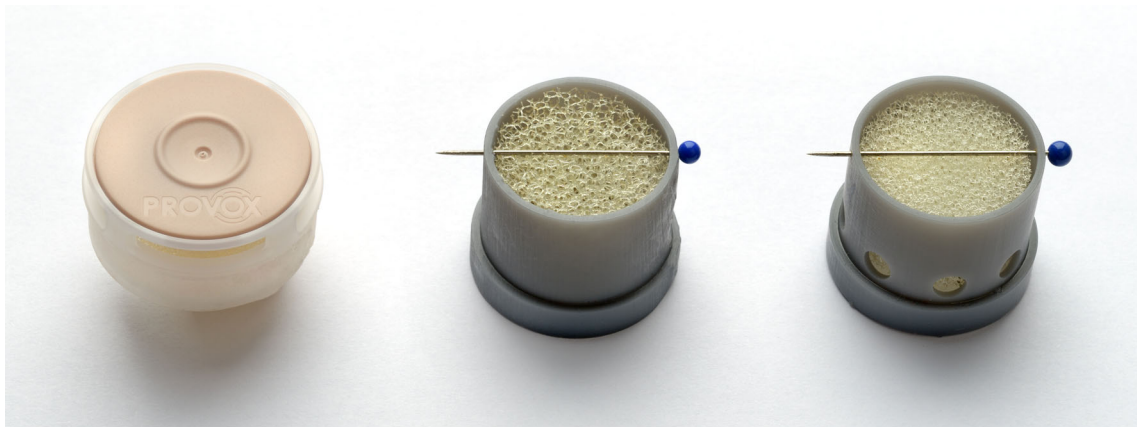
FIGURE 1 The photo shows, from left to right, the original HME cassette of both the XF and XM with speaking valve (pink lid), the 3D-printed (FormLabs, Form2) closed cassette with inserted XF foam and the 3D-printed (FormLabs, Form2) cassette with bypass on the tracheal side, with inserted XM foam (note the difference in pore size between the two different foams). A speaking valve was not included in the 3D printed cassette designs to simplify the prototyping and to limit the scope of this proof of principle study to only the effect of the bypass. The thicker cylinder at the base of the 3D-printed cassettes is used to connect them to the measurement set-up (spirometer). HME, heat and moisture exchanger; XF, lower resistance/lesser humidification HME; XM, high resistance/high humidification HME [Color figure can be viewed at wileyonlinelibrary.com]
