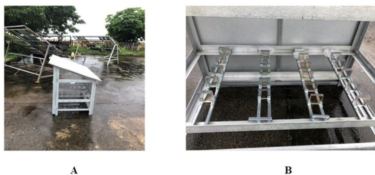
Figure 2. The placement of samples at the testing station, Tropical Center, Nha Trang, Vietnam. (A)—concrete platform with installations for placing organic glass samples; (B)—installation with placed samples.
