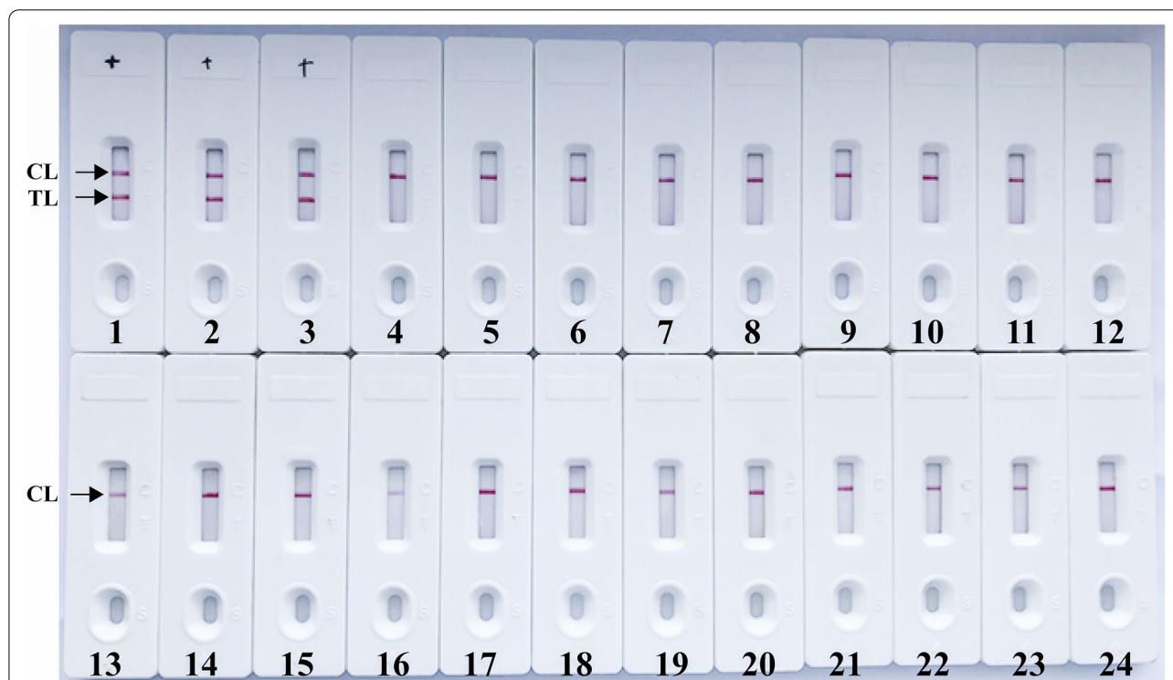
Fig. 6 Analytical specificity of B. pseudomallei -MCDA-NB assay using different bacterial strains. The B. pseudomallei -MCDA-NB was evaluated using different genomic DNA templates. Biosensor 1, B. pseudomallei (BPC006); biosensor 2, B. pseudomallei (BP053); biosensor 3, B. pseudomallei (BP069); biosensor 4, B. thailandensis ; biosensor 5, B. cepacia ; biosensor 6-23, Pseudomonas aeruginosa ; Klebsiella pneumoniae ; Staphylococcus aureus ; Bacillus cereus ; Staphylococcus epidermidis ; Candida tropicalis ; Candida albicans ; Staphylococcus saprophyticus ; Enterotoxigenic E. coli ; Salmonella ; Shigella flexneria ; Listeria monocytogenes ; Streptococcus pneumoniae ; Staphylococcus suis ; Enterococcus faecalis ; Enterococcus faecium ; Vibrio parahaemolyticus ; Stenotrophomonas maltophilia ; biosensor 24, negative control (DW)
