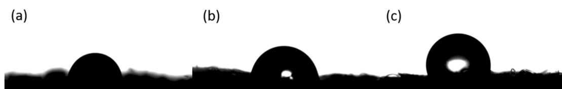
Figure 6. Water contact angle in air above the lower critical solution temperatures (LCSTs) of (a) P1, (b) P2, and (c) P3 samples.
