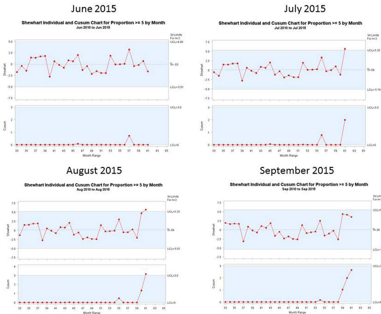
Figure 3. CUSUM and Shewhart control chart output for Jurisdiction 2, June to September 2015 (3-SD threshold exceedance occurs during July [Shewhart] and August [CUSUM and Shewhart], 2015).
