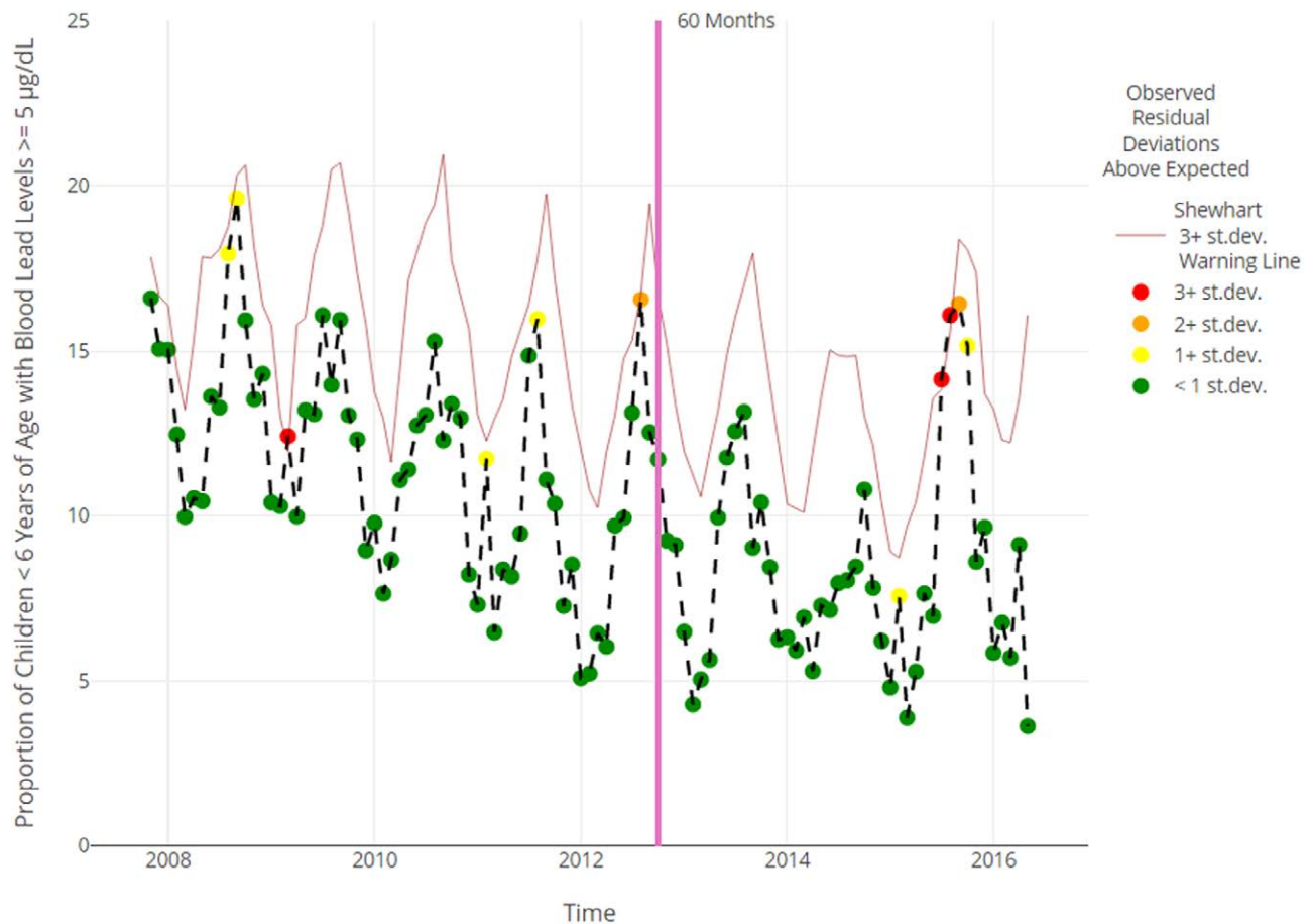
Figure 4. CUSUM and Shewhart control chart output for Jurisdiction 2 using R-Shiny Application, January 2007 to May 2016 (3-SD threshold exceedance occurs during July and August 2015)
