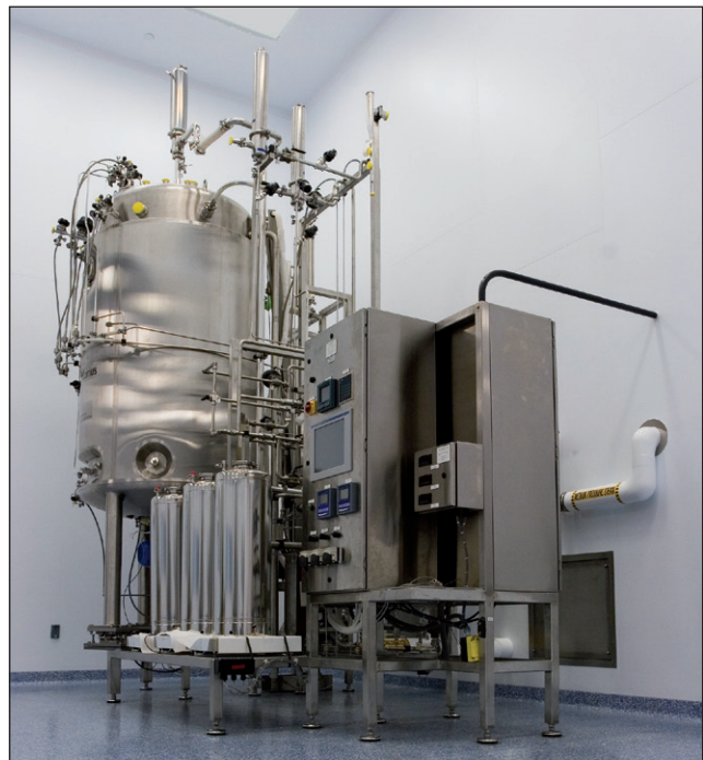
Figure 4-3 Typical bioreactor used in vaccine manufacturing.
