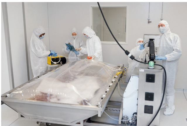
Figure 4-4 Single-use bioreactor for cell culture (courtesy GE Healthcare).
