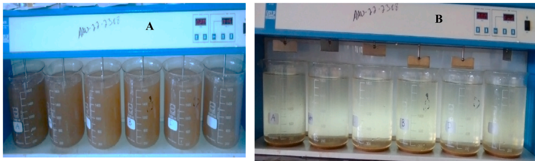
Fig. 2. Moringa Oleifera seed coagulation and settling (A, moringa slurry and coagulating; B, Settling).
