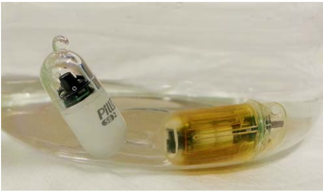
Fig. 5 Floating characteristics of Pillcam SB2 (left) and Smartpill (right) submerged in 400 mL sterile water for irrigation.
