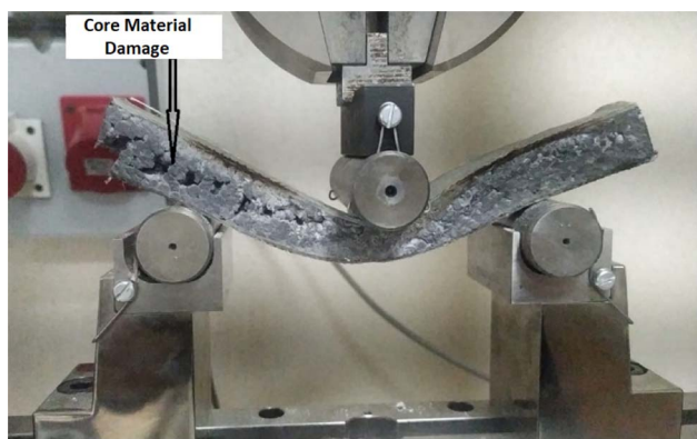
Fig. 12 Compression test view of EPS 8-300 foam core specimen.
