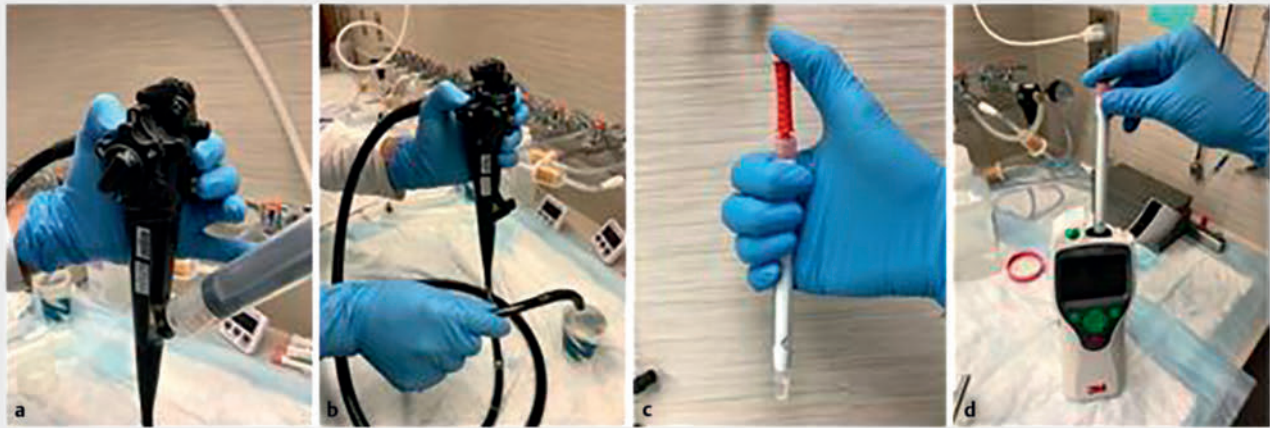
► Fig. 2 ATP sampling protocol. The suction/biopsy channel is purged with air and then flushed with 40 mL of water. The channel is then purged again and the effluent is collected in a disposable cup. The distal portion of the ATP stick is submerged in the sample, and then returned to its holder and depressed to activate the bioluminescence reaction. This reaction is then quantified by the luminometer in the form of relative light units (RLUs).
