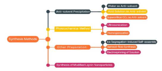
Figure 4. Overview of the synthesis and modification methods of nano-lignin.
