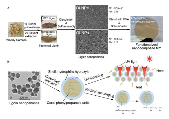
**Figure 7.** (a) Synthesis of lignin nanoparticles/PVA composite film. (b) Proposed mechanism for UV-shielding and antioxidant activity using lignin nanoparticles as the functional additive. Reprinted from Tian et al. [133].
