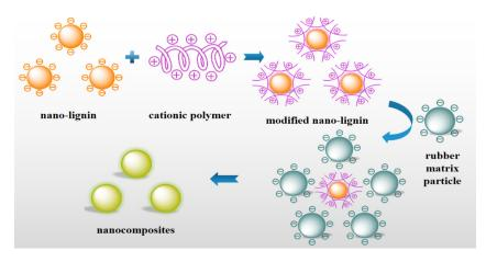
Figure 6. Preparation of nanocomposites of modified nano-lignin and rubber matrix.
