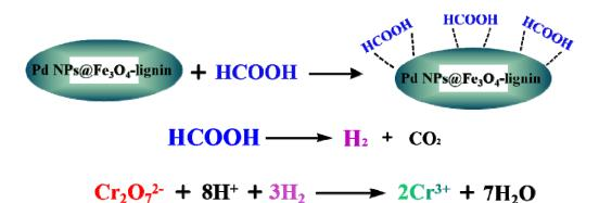
Scheme 2. The reduction of Cr(VI) by using Pd NPs@Fe<sub>3</sub>O<sub>4</sub>-lignin.
