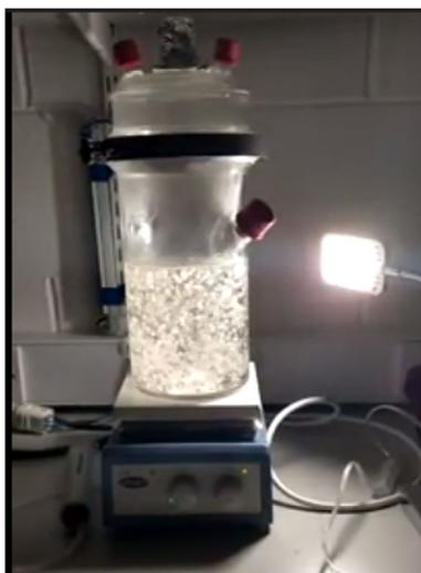
**Figure 1.** Photograph of stirred tank photobioreactor containing CuS–Bio NBs.
