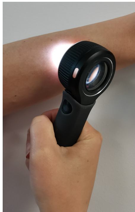
Figure 2. Photograph of a handheld dermoscopic sensor with non-polarized and polarized light, which is used by dermatologists during their clinical examination. The dermatoscope shown in the figure is produced by Dermoscope DermLite DL4, 3GEN Inc., San Juan Capistrano, CA, USA.
