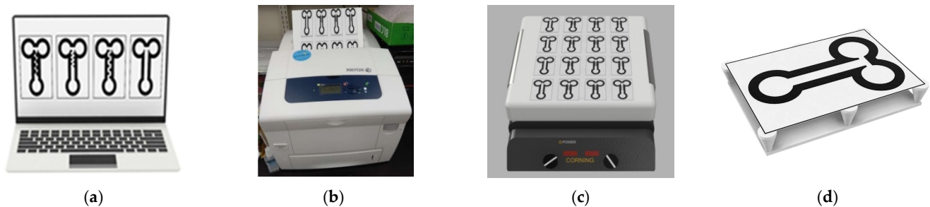
Figure 2. Schematic flowchart of the fabrication process. (a) Design, (b) wax printing, (c) baking, and (d) cutting.
