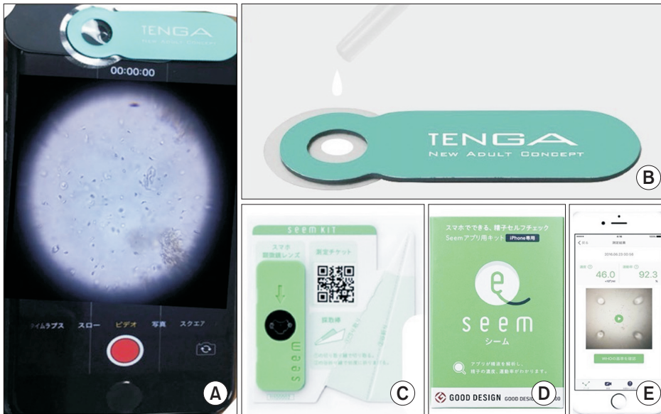
Fig. 4. Men's Loupe (Tenga Health Care) device and smartphone-based SEEM kit. (A) Men's Loupe 0.8 mm diameter ball lens microscope attached to smartphone. (B) Technique for loading semen sample into plastic jacket of ball lens microscope. (C) Magnifying lens semen analysis device with QR code sheet to download the application for operating. (D) Instructions of kit for use. (E) Screenshot of sample test results with concentration and motility.
