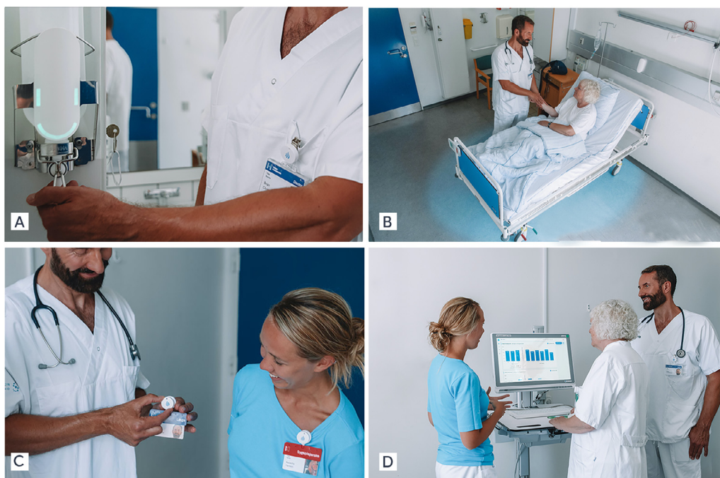
Fig 1. The Sani nudge hygiene system: (A) Sensor on a dispenser registering the number of alcohol-based hand rubbing events and displaying a nudge (green smiley) as a reward when a sanitization is performed. (B) The patient zone (illustrated with blue) created by the sensor near the head of the patient bed. (C) An anonymous sensor on the name badge of each health care worker. The sensor is coded according to staff profession (doctors and nurses). (D) Data captured by the sensors are sent to a secure cloud-based server and stored at the device level. Weekly performance data on group level is sent to the infection control nurses and ward managers, shown at staff meetings and put up on bulletin boards.
