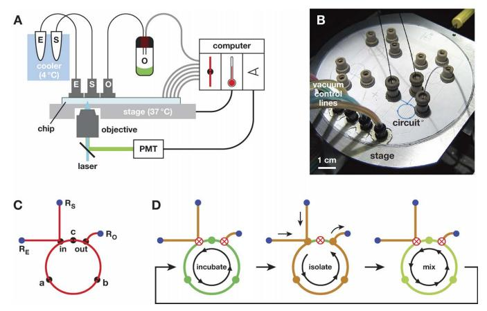
Figure 1. Microfluidic Evolution System
