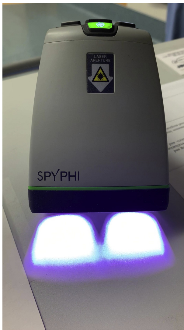
VIDEO 1. A handheld probe via a sterile sleeve is used for image acquisition intraoperatively. It emits infrared rays, which excites indocyanine green fluorescence. Video available at: https://www.jtcvs.org/article/S2666-2507(21)00178-4/fulltext .
