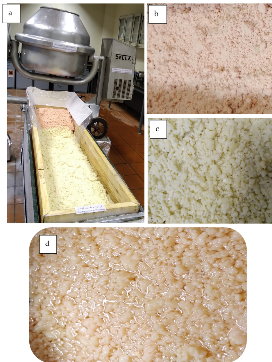
Figure 3. Microcapsules' fabrication process: (a) the mechanical mixer used to blend polymeric matrix, (b) the air-dried alginate-based encapsules (ABEs), (c) the air-dried guar gum-based encapsules (GGBEs), and (d) immersing ABE in essential oil solution.
