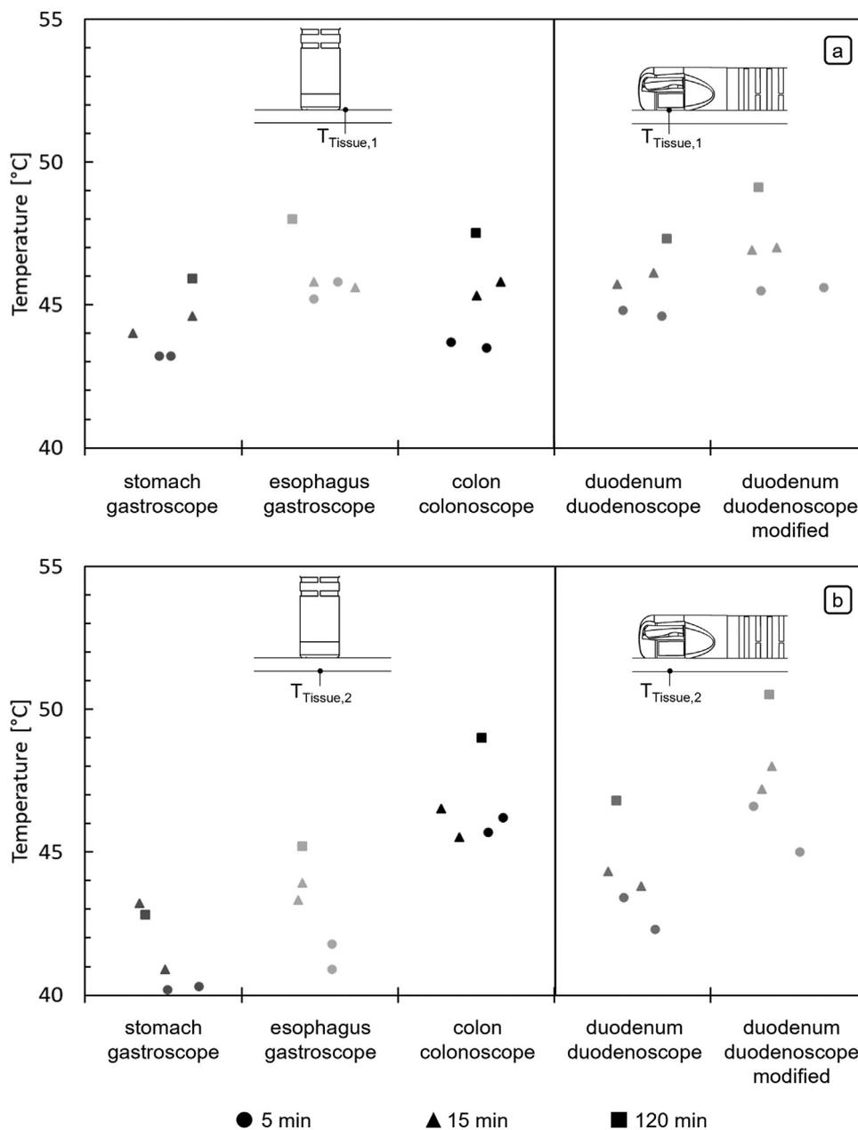
**Figure 3.** Maximum tissue temperatures measured. (A) Temperature at tissue surface next to the endoscope tip ( $T_{Tissue,1}$ ). (B) Temperature at the lower side of the tissue underneath the endoscope tip ( $T_{Tissue,2}$ ).
