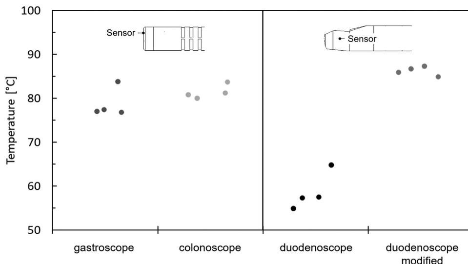
**Figure 1.** Absolute maximum temperatures at endoscope contact points. Four measurements per endoscope are individually shown. The sensors at the tissue-contacting area are shown for all endoscopes; that is, for gastroscope and colonoscope, the temperatures of the sensor at the light-emitting diode are shown, and for the duodenoscopes, the results of the sensor at the lateral side are shown.
