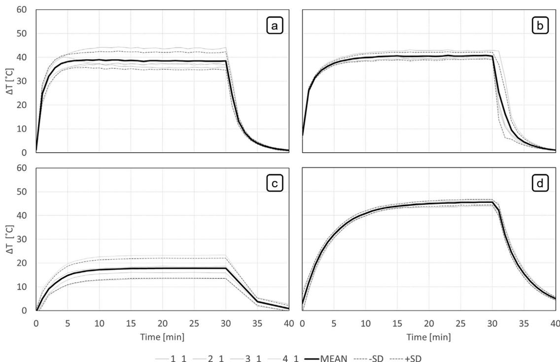
**Figure 2.** Endoscope tip temperature increase in a benchtop setting. Within the climate chamber, temperature change ( $\Delta T$ ) relative to chamber temperature. (A) Gastroscope, sensor at light-emitting diode (LED). (B) Colonoscope, sensor at LED. (C) Duodenoscope, sensor at lateral side (objective). (D) Modified duodenoscope, sensor at lateral side (objective). Mean (SD) is displayed as well as single experiments ( $n = 4$ ).
