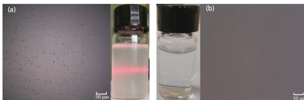
Fig. 8 Photographs and optical microscopy images of O/W emulsions (a) and the permeate (b) separated by the SiC hollow fiber membranes.
