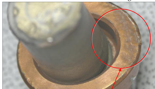
Obvious plastic deformation on the nut
