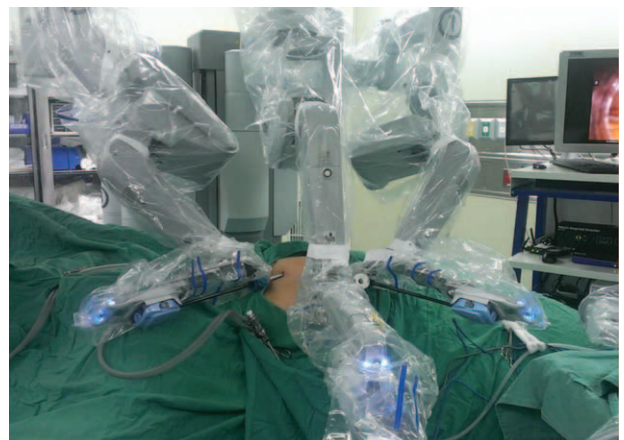
FIGURE 3. Docking the robot: The robot was docked over the ipsilateral shoulder at a 30° angle from the patient's spine.
